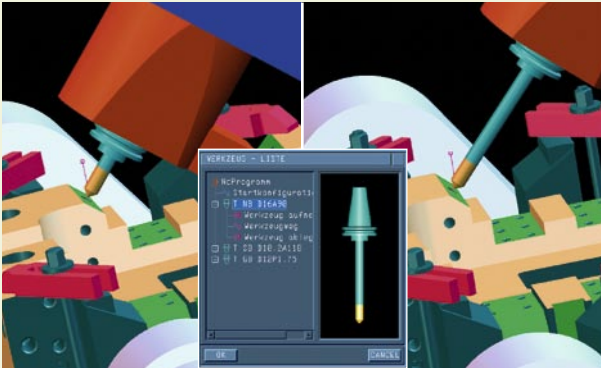
Eliminating collisions by inserting a longer tool
