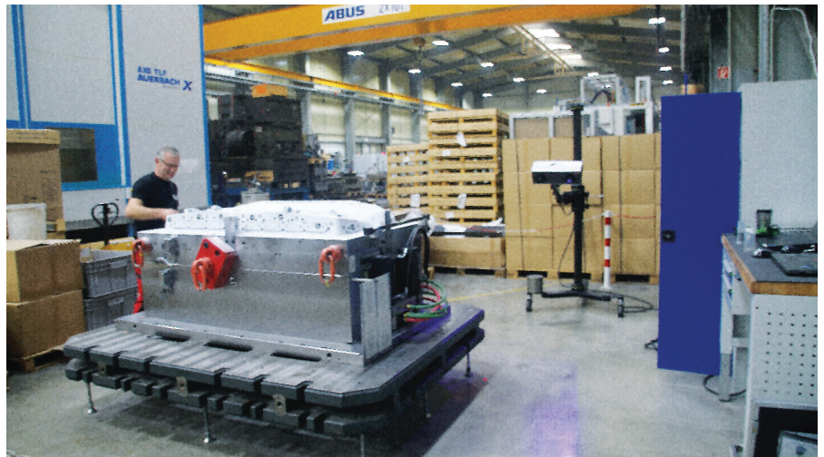
Optical instrumentation for quality assurance is now a part of daily life for large die manufacturers. The data are carefully recorded, and not just for the customer.
