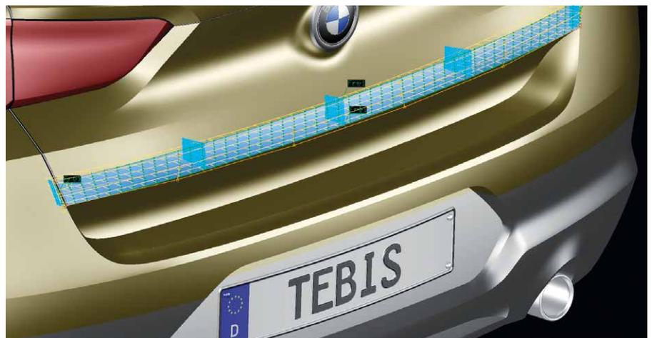
*Theoretical edges are automatically retained in Tebis during reverse engineering and surface modeling. Special functions are available in the software to quickly generate theoretical edges.*
